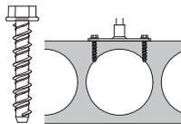
Drilling depth for concrete at least 60 mm (Ø 8 mm),
